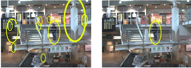
Fig. 6. **Data fusion.** *Left:* Result of a person detection method with a high rate of false-positives. *Right:* Result of the fusion process. Here, the results of motion detection, background segmentation and person detection are fused which, in that case, eliminates all false-positives.
