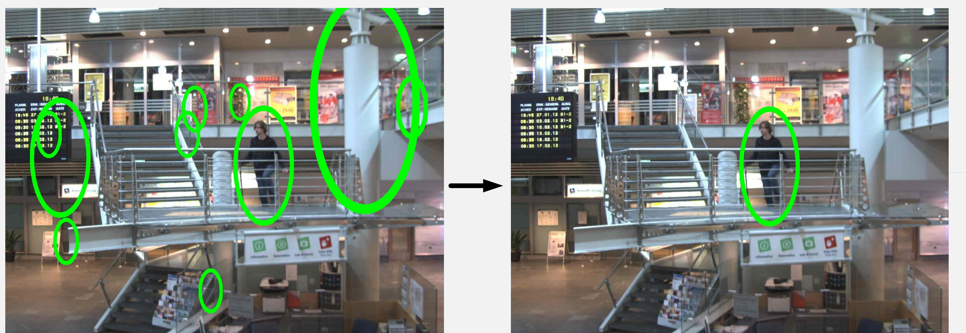
Fig. 3: Data Fusion. Left: Result of a person detection method with a high rate of false-positives. Right: Result of the fusion process. Here, the results of person detection, background segmentation and motion detection are fused which, in that case, eliminates all false-positives.
